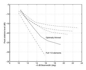
Figure 2. Sidelobe level as a function of beamwidth for several weight-optimized uniform sidelobe cases: 112 element full array (dash-dot line) and three realizations of random thinning to 64 elements (dashed lines). The best result is obtained for a layoutoptimized 62 element thinning (solid line).
